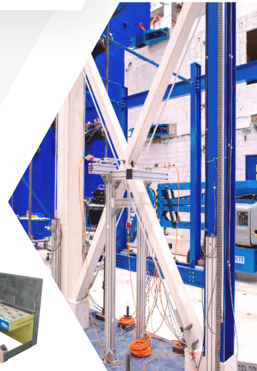
PROMATECT®-H board seismic testing for the European EQUFIRE project
